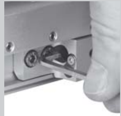
Adjustment of the absorption screw.
