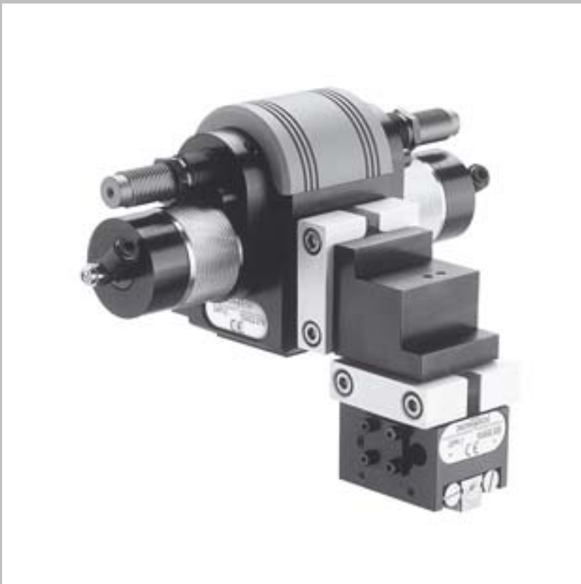
Robust transfer module; Precision Parallel Gripper GPP, perpendicular to axis of rotation, with angle adapter WA mounted on Rotary Drive DAPI-2; internal air flow permitted. Elimination of moving hoses.
