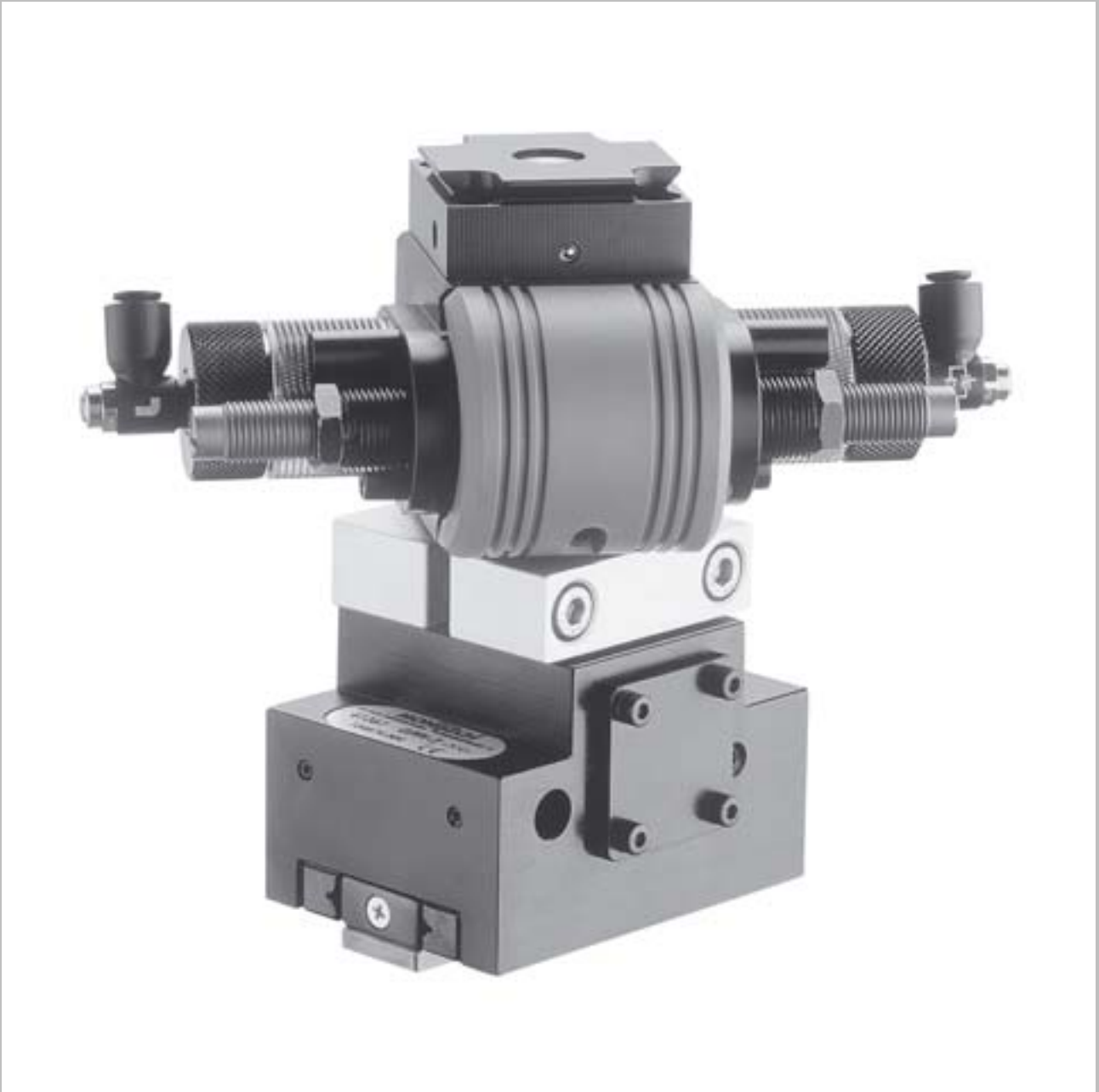
Rotary Drive with internal air flow; Precision Parallel Gripper GPP fitted, supplied internally with compressed air by Rotary Drive DAPI-1; all moving hoses are eliminated.
